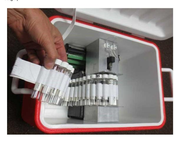
The "Undercap Unfiller" is a chamber that evacuates Exetainers without puncturing the septum. The vial is evacuated with the cap loose then the cap is tightened while still in the vacuum chamber. Vials are evacuated in seconds instead of minutes as with using a needle. You can use a nut driver or similar tool to tighten the caps to save wear and tear on your fingers
