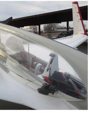
Bandolero<sup>™</sup> autosampler mounted in the passenger seat of a Long-EZ aircraft for landscape scale sampling and plume sampling.
